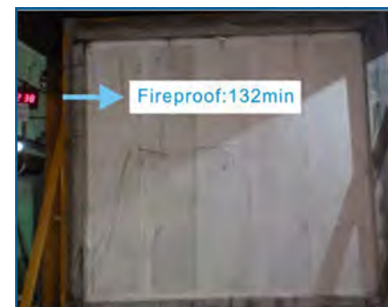
The unexposed surface of the specimen after the test
